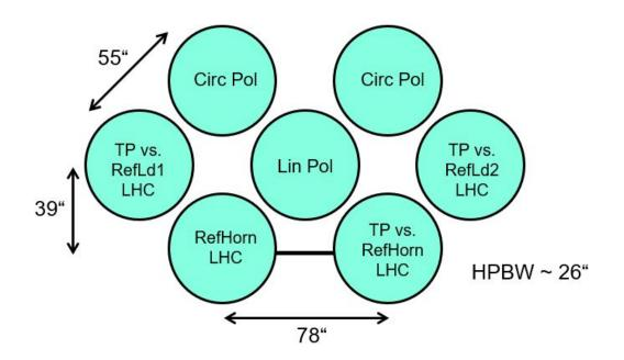
Horn layout of the7 beam 9mm receiver with beam spacing on sky indicated
