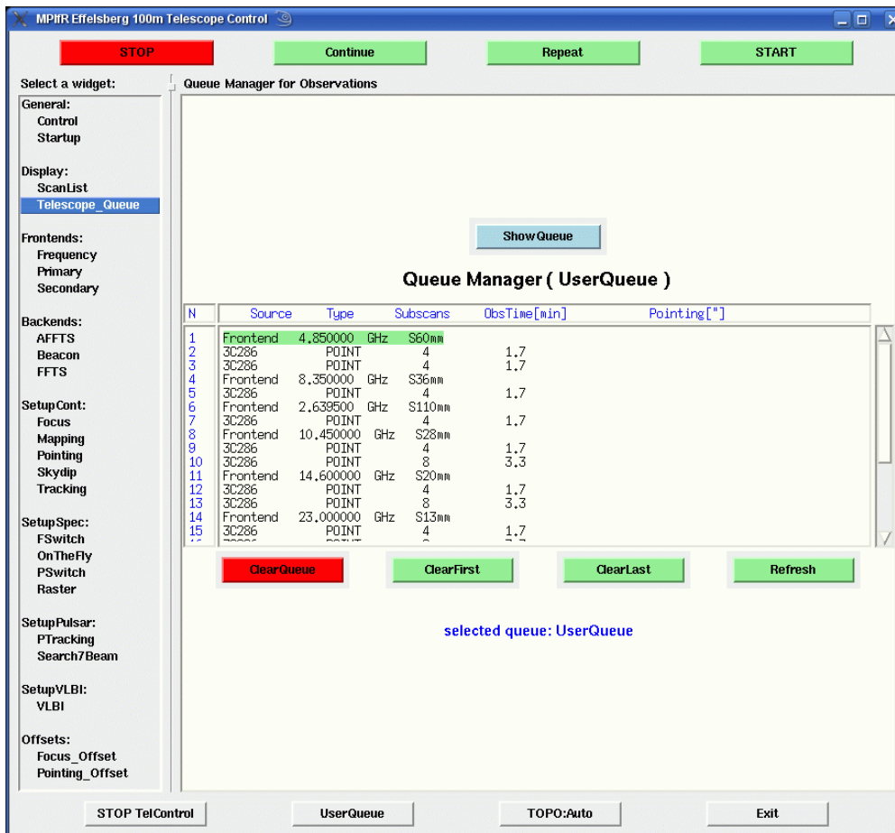
Figure 3: Top: The ScanList shows the most recent 100 scans with some basic information about observing modes and receivers used. Bottom: Example for a queue filled with pointing scans using different secondary focus receivers.
