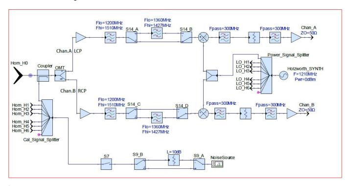
**Detail Receiver Block Diagram**
