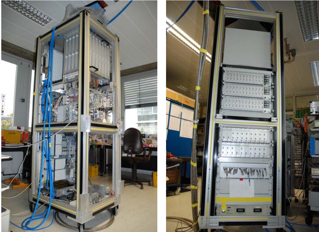
Figure 1 9mm 7beam receiver during assembly and tests in the lab
