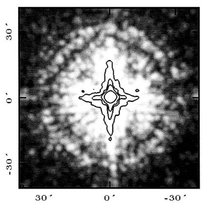
Fig. 3: Antenna pattern at 11.7 GHz slightly convolved to 2' in order to enhance the contrast of the weak outer sidelobe structures. The dynamic range is about 60 dB.
