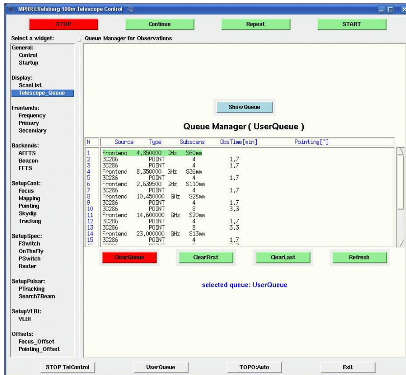
Figure 3: Top: The ScanList shows the most recent 100 scans with some basic information about observing modes and receivers used. Bottom: Example for a queue filled with pointing scans using different secondary focus receivers.
